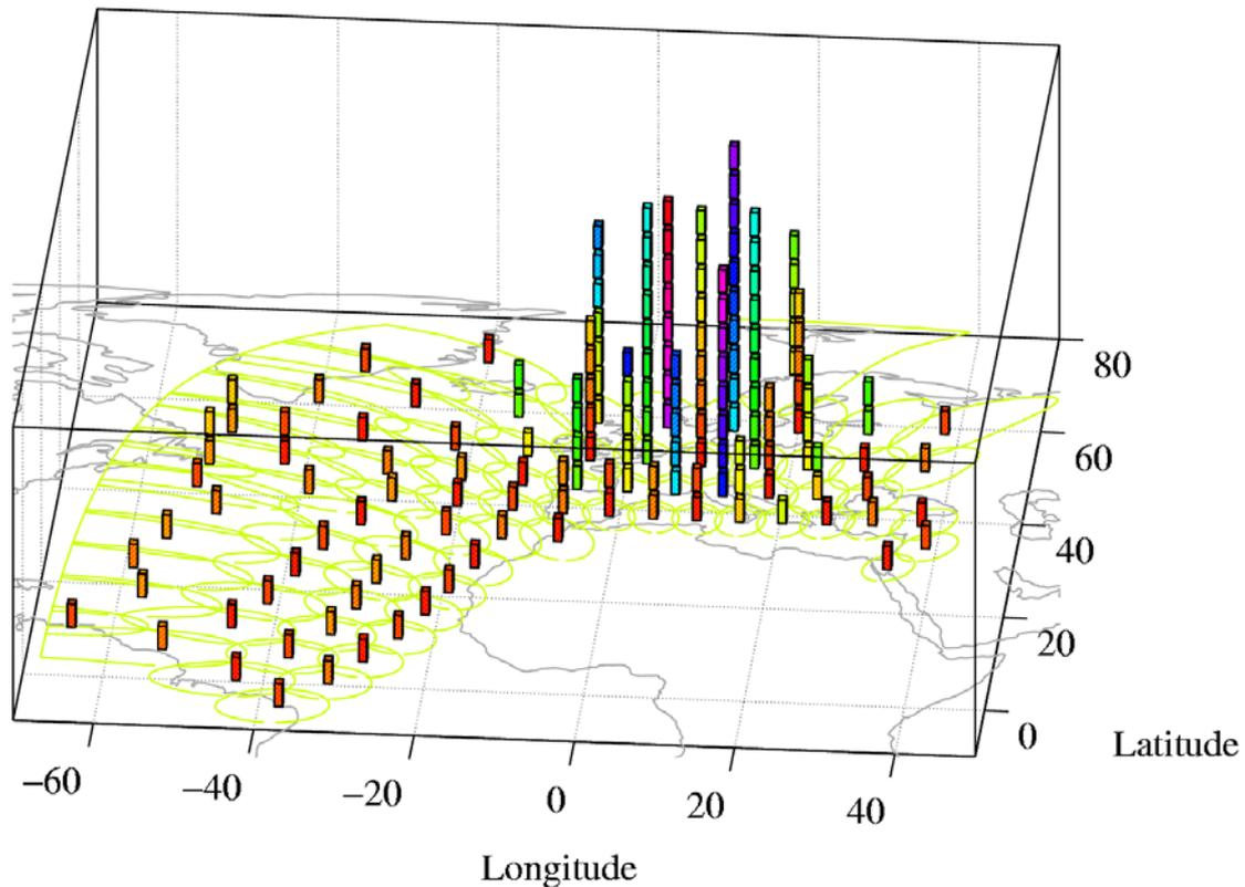
Figure 8: Optimized aircom traffic and carrier assignment for the ABATE scenario
