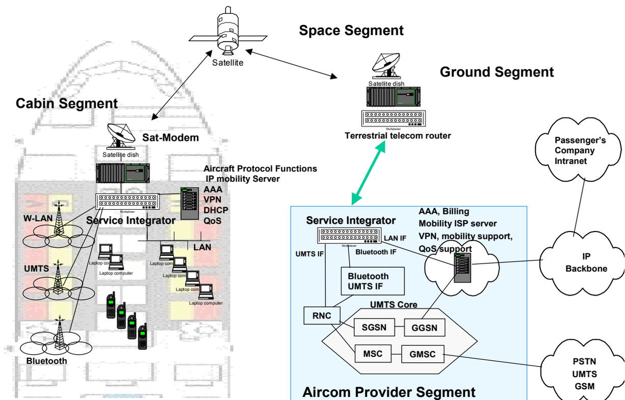
Figure 1: WirelessCabin network architecture
