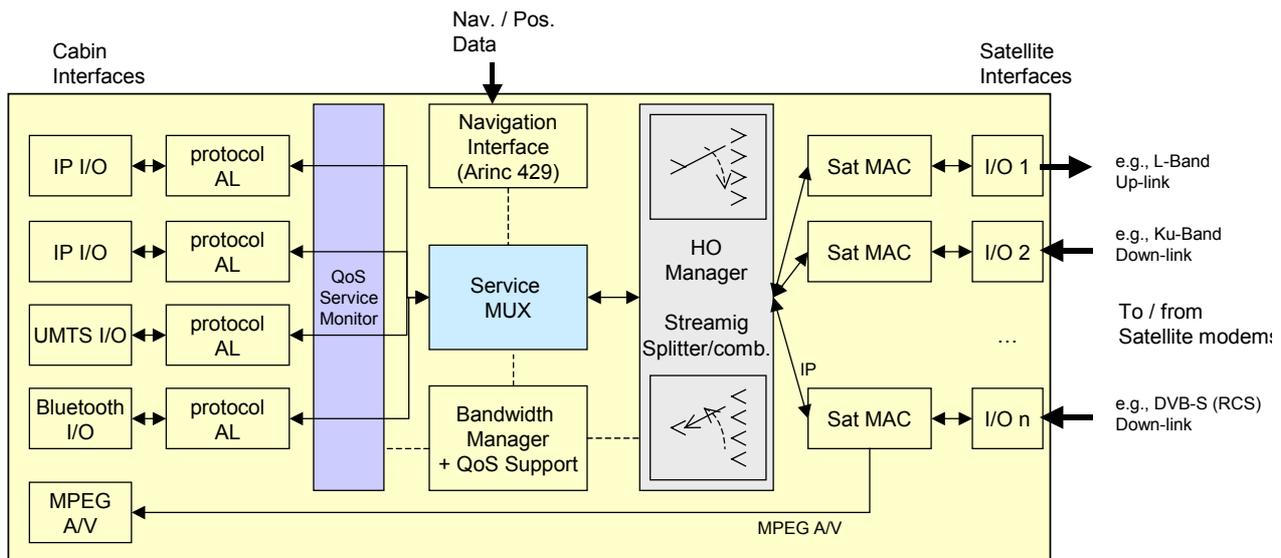
Figure 4: Service Integrator: core of the Collectively Mobile Heterogeneous Network
