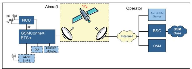
The BTS+ GSM Base Transmitter Station and Controller is connected via satellite to a GSM operator.
